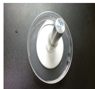
Figure 4. AUL unit in a soaking dish. [Color figure can be viewed in the online issue, which is available at wileyonlinelibrary.com .]
