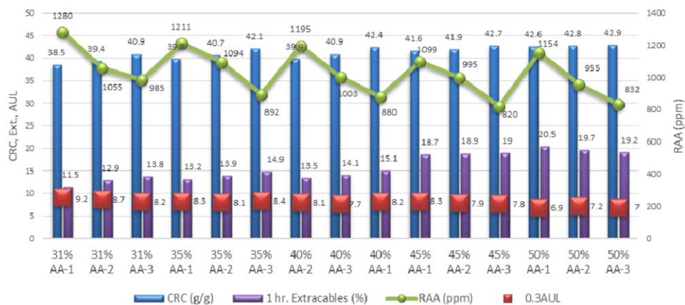
Figure 7. Measured polymer properties at different acid contents (free-radical solution polymerization). The conditions for AA-1 were 150-ppm \text{H}_2\text{O}_2 , 150-ppm \text{C}_6\text{H}_8\text{O}_6 , and 75-ppm (\text{NH}_4)_2\text{S}_2\text{O}_8 . The conditions for AA-2 were 175-ppm \text{H}_2\text{O}_2 , 175-ppm \text{C}_6\text{H}_8\text{O}_6 , and 100-ppm (\text{NH}_4)_2\text{S}_2\text{O}_8 . The conditions for AA-3 were 225-ppm \text{H}_2\text{O}_2 , 225-ppm \text{C}_6\text{H}_8\text{O}_6 , and 125-ppm (\text{NH}_4)_2\text{S}_2\text{O}_8 . [Color figure can be viewed in the online issue, which is available at wileyonlinelibrary.com .]
