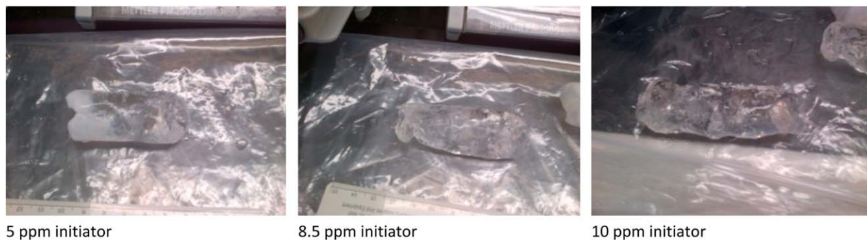
Figure 10. Images of a polymer made with 31% acrylic acid. [Color figure can be viewed in the online issue, which is available at wileyonlinelibrary.com.]
